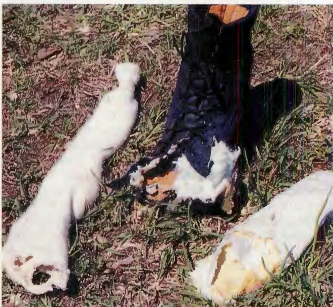
(below) Effects on boot and simulated foot by two ounces of HE are graphic: Almost half the boot is destroyed. In contrast, the sock (filled with wet sand and half a dozen wooden stakes to simulate human bones and protected by Davis' Kevlar pad), though slightly damaged, remained intact. In a real AP mine blast with this measure of Kevlar protection, a man's foot would almost certainly be broken, but victim wouldn't lose the foot, as is usually the case with small AP mines like the Russian PMN.
