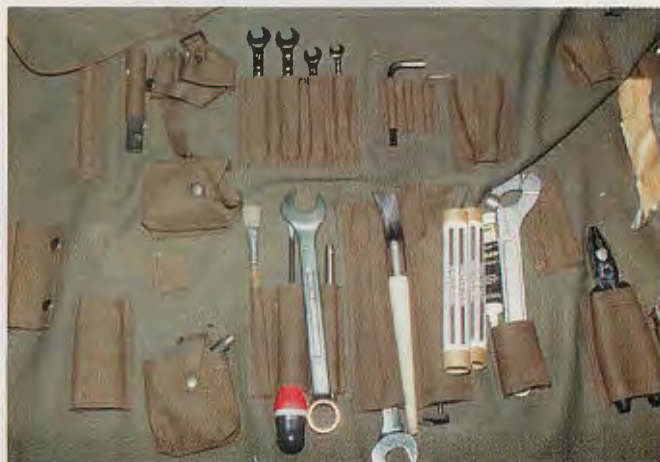
Ever meticulous about providing operators and armorers with specialized tools and equipment to properly maintain its weapons, FN supplies this gunner's kit — just a small part of the armorer's tool roll that comes with the M3M system.
