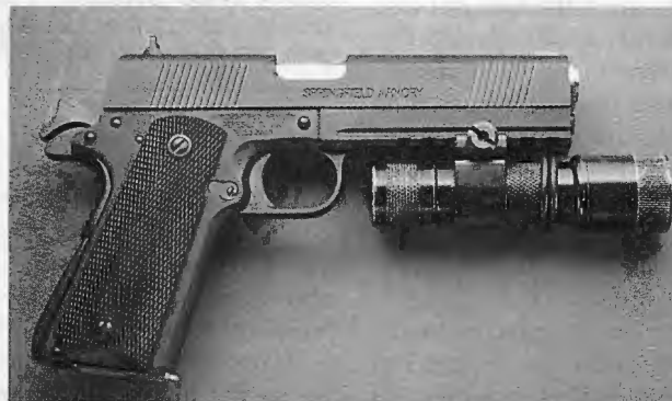
The author used a Weaver-style scope ring and mount, together with his Sure-Fire Model 6P flashlight, to create this tactical-lamp-equipped home-defense weapon.
