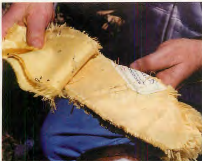
Though blown ragged, a detailed inspection of the inner Kevlar sheets of the pad show no evidence of damage.
