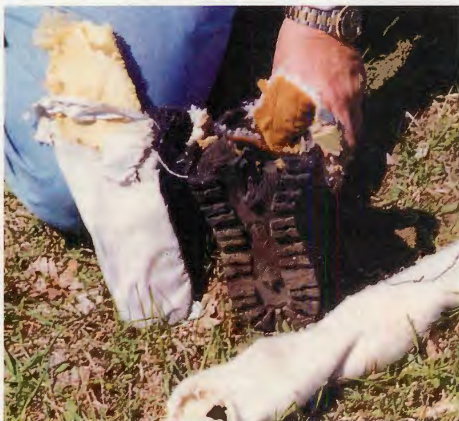
Close-up of the half-destroyed boot shows that sock filled with sand and the layered Kevlar pad came out of the blast almost intact.
