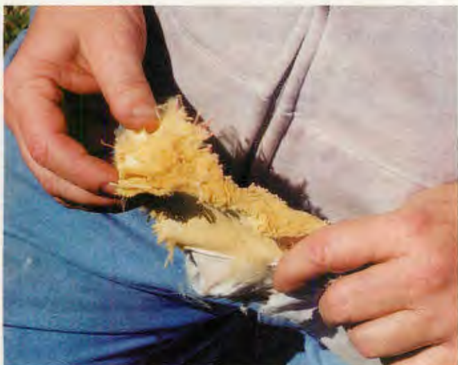
The 40-layered Kevlar pad is light, thin and pliable. After four months in one of Davis' boots, it was little the worse for wear because Kevlar quickly conformed to individual foot contours.
