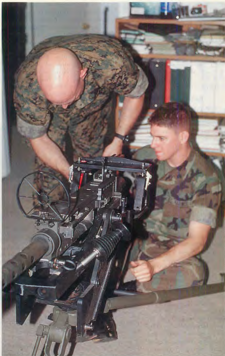
he M3M is a "system" for machine gunnery, consisting of the gun itself, mated with this very cleverly designed soft-recoil mount. Here we see the mount affixed to standard GI M3 tripod for ground-use trials. A special adapter is also provided to allow use of the normal traversing and elevating mechanism for the M2HB. Note how this cradle is set up with the red firing handle on the right side.
