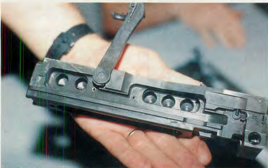
Milled cavities and holes lighten the M3M's bolt for faster cycling without as much weight to deal with mechanically, in punishing start/stop action.
